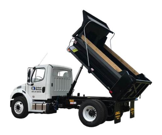
Spring loaded crank type tarp cover
