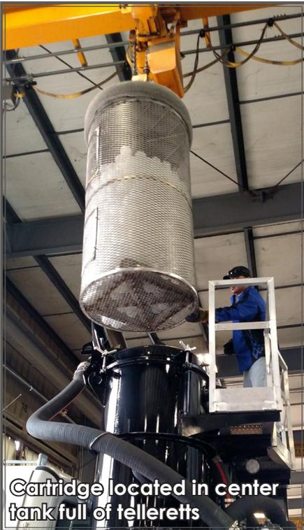
Cartridge located in center tank full of telleretts
