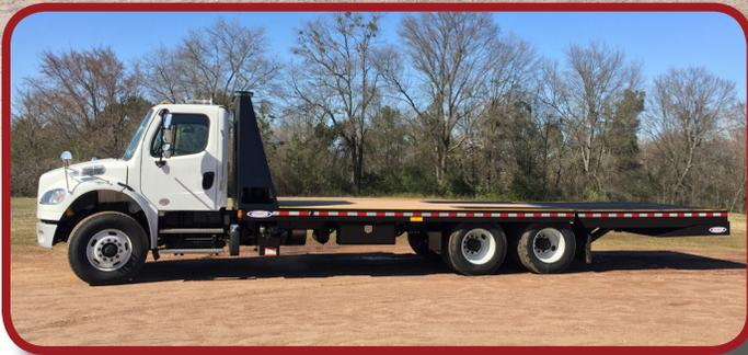
The Ledwell Hydratail Truck is a great option to haul equipment, especially in tight spaces found in urban areas. This piece of equipment features the same tail as the popular Ledwell Hydratail Trailer, requiring significantly less ground to load. The Hydratail Truck bed sits directly on the chassis frame, allowing
